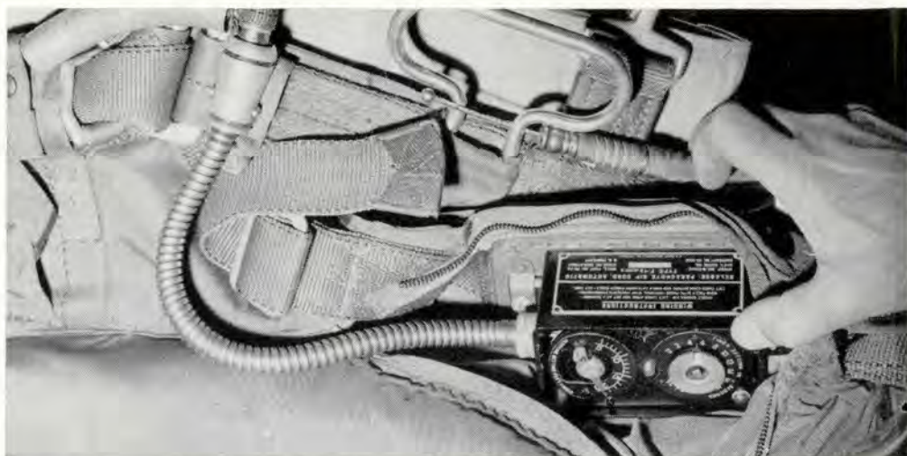
The automatic parachute ripcord release is one step in the right direction. Another fairly new development being tested is the supine seat with seat bucket for protection and booms for stabilization.
